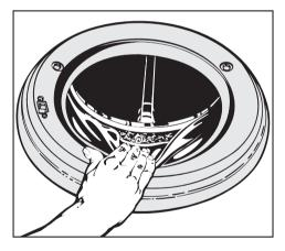
Check the folds in the door seal for any small articles e.g. buttons which might be lodged there.
